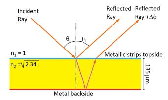
The metallic strips must be placed 45 degrees with respect to the plane of polarization of the incident wave, then half of the incident power will be reflected on the strips surface and the other half will be reflected by the metal backside surface.
